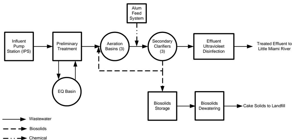
**Figure 1 – Flow Diagram for Greene County Sugarcreek WRRF**
