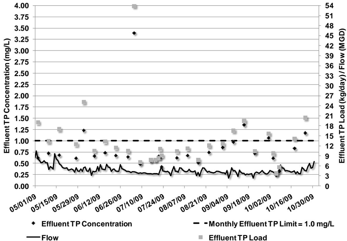
**Figure 5 –Effluent TP concentration and load and wastewater flow for May through October 2009**
