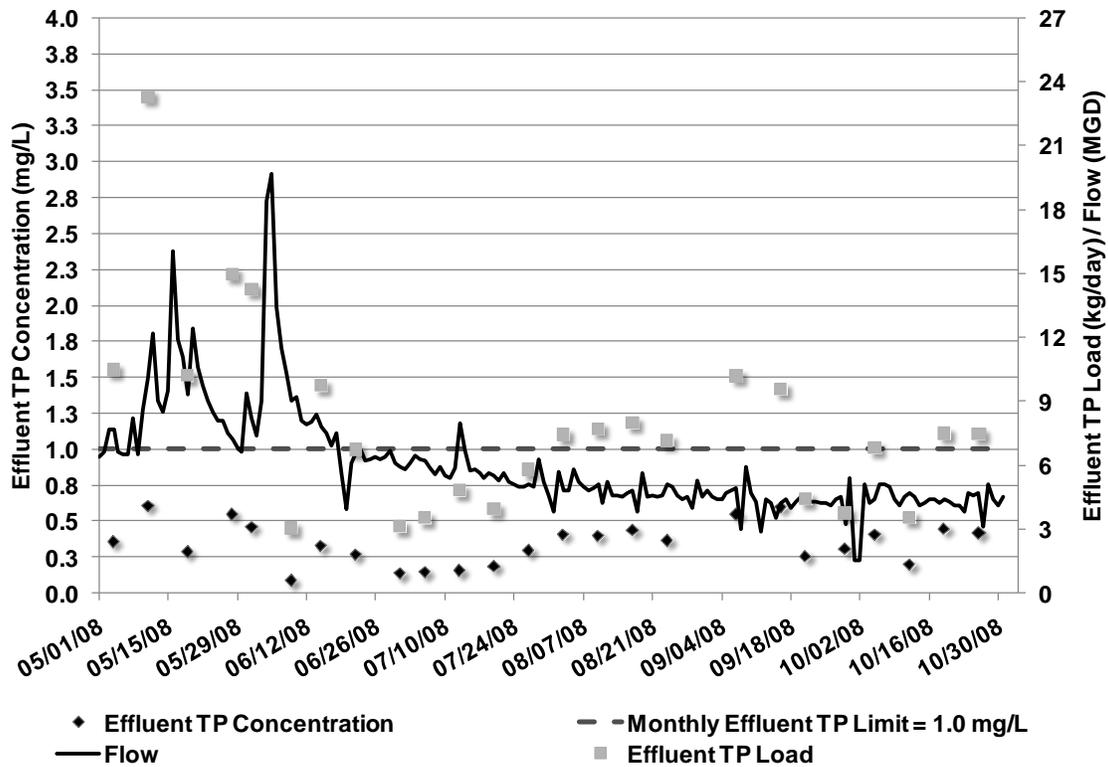
**Figure 4 –Effluent TP concentration and load and wastewater flow for May through October 2008**
