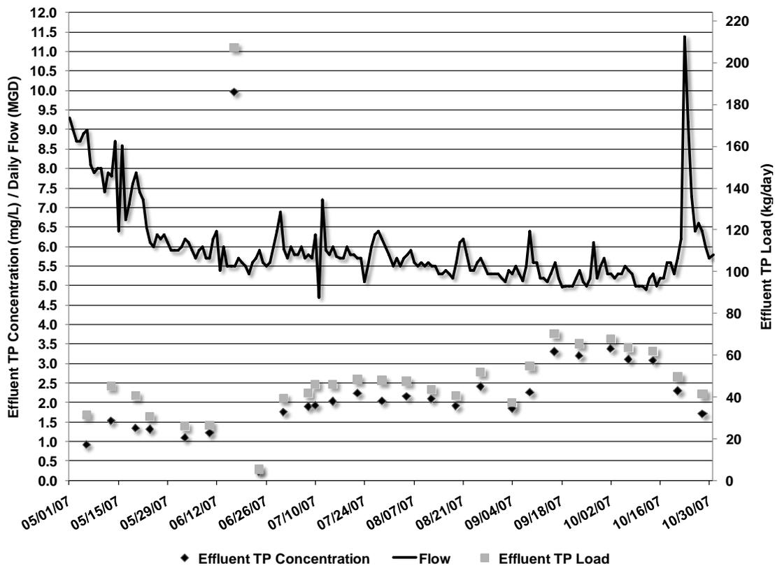
**Figure 3 –Effluent TP concentration and load and wastewater flow for May through October 2007**
