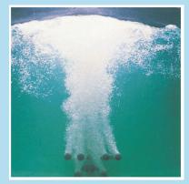
Stationary diffusers alone create a vertical updraft of water, increasing bubble rise rate, reducing contact time, and leading to a coalescence of bubbles that reduces available O<sub>2</sub> surface area for low oxygen transfer.
