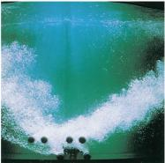
By moving the water horizontally over stationary diffusers, the CSR's rotating diffusers eliminate the updraft problem created by stationary diffusers alone. The combination of rotating and stationary diffusers can greatly increase aeration capacity for higher basin loadings.
