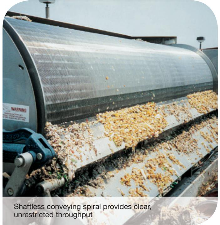
Shaftless conveying spiral provides clear, unrestricted throughput
